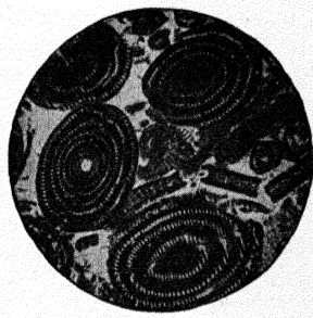
FIG. 14.—Microscopic section of limestone containing foraminifera; from India (magnified about \frac{1}{2} ).
